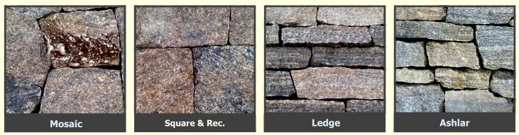
**Thin Stone Veneer** is the sawn facings of traditional "full bed" building stone veneer. Whereas traditional building stone veneer typically ranges in thickness (depth) from 3" to 5" and requires a bearing shelf, thin veneer products vary in thickness between  $\frac{3}{4}"$  and  $\frac{11}{4}"$  and do not require any special foundations. 90° angle cuts taken from the interior of full bed cutting stock produce thin veneer corners that help conceal the overall material depth.
