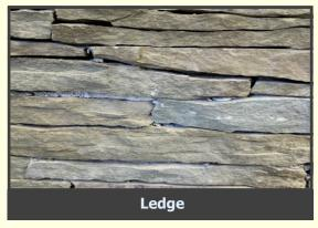
**Thin Stone Veneer** is the sawn facings of traditional "full bed" building stone veneer. Whereas traditional building stone veneer typically ranges in thickness (depth) from 3" to 5" and requires a bearing shelf, thin veneer products vary in thickness between ¾" and 1¼" and do not require any special foundations. 90° angle cuts taken from the interior of full bed cutting stock produce thin veneer corners that help conceal the overall material depth.
